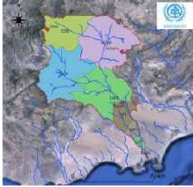
Figure 18. Boundaries of Watersheds Contributing to Flash Flood Risks in the Tuban Delta
