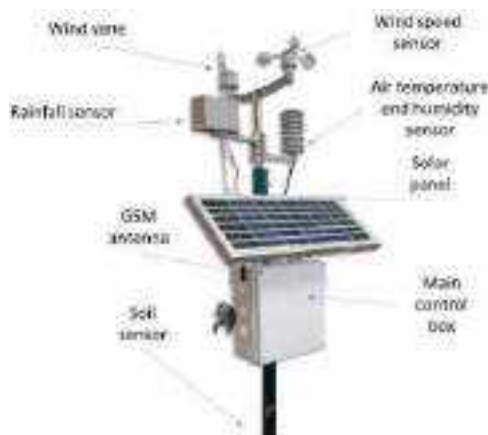
Figure 4. Scheme of an agro-meteorological station (Source: UNDP 2021 )
