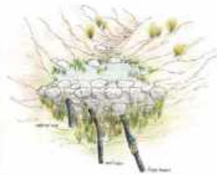
FIGURE 3. STONE RETAINING WALL OF THE MINI DAMS
