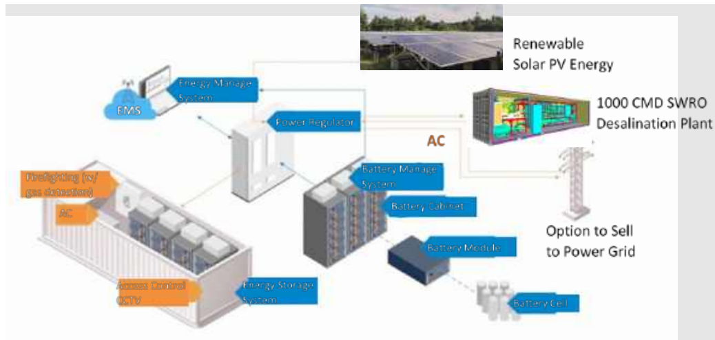
Figure 10. Illustrative diagram of a solar PV energy system attached to the SWRO desalination plant
