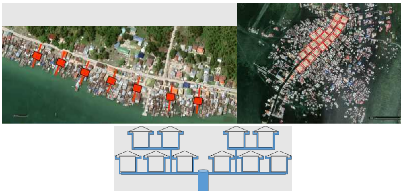
Figure 18. Illustrative example of communal rainwater harvesting clusters
