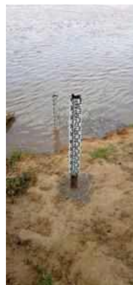
Water level gauge
