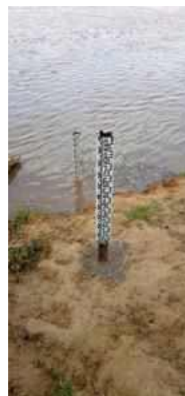
Water level gauge
