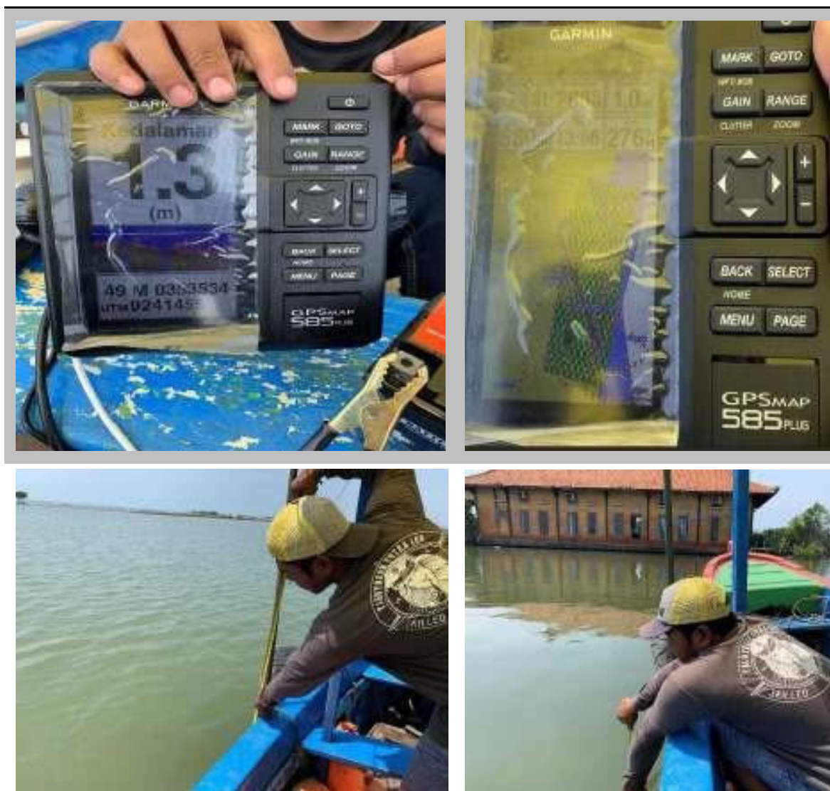
5.1.1.46 Figure 3.27 Documentation of bathymetric measurement and manual checking Table 3.15 Snippet of actual depth checking data for
