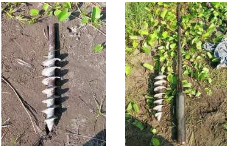
Figure 6.4 Hand boring tools used
