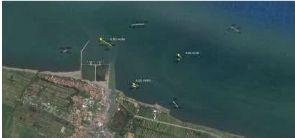
5.1.1.94 Figure 9.20 Vector of Surface Current speed in Batang Waters during the Low Tide condition (BPPT, 2015)
