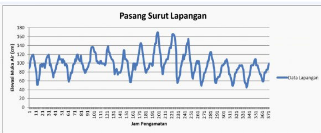
Figure 5.11 Tidal elevation graph based on 15 days of observations with reference to MSL field
