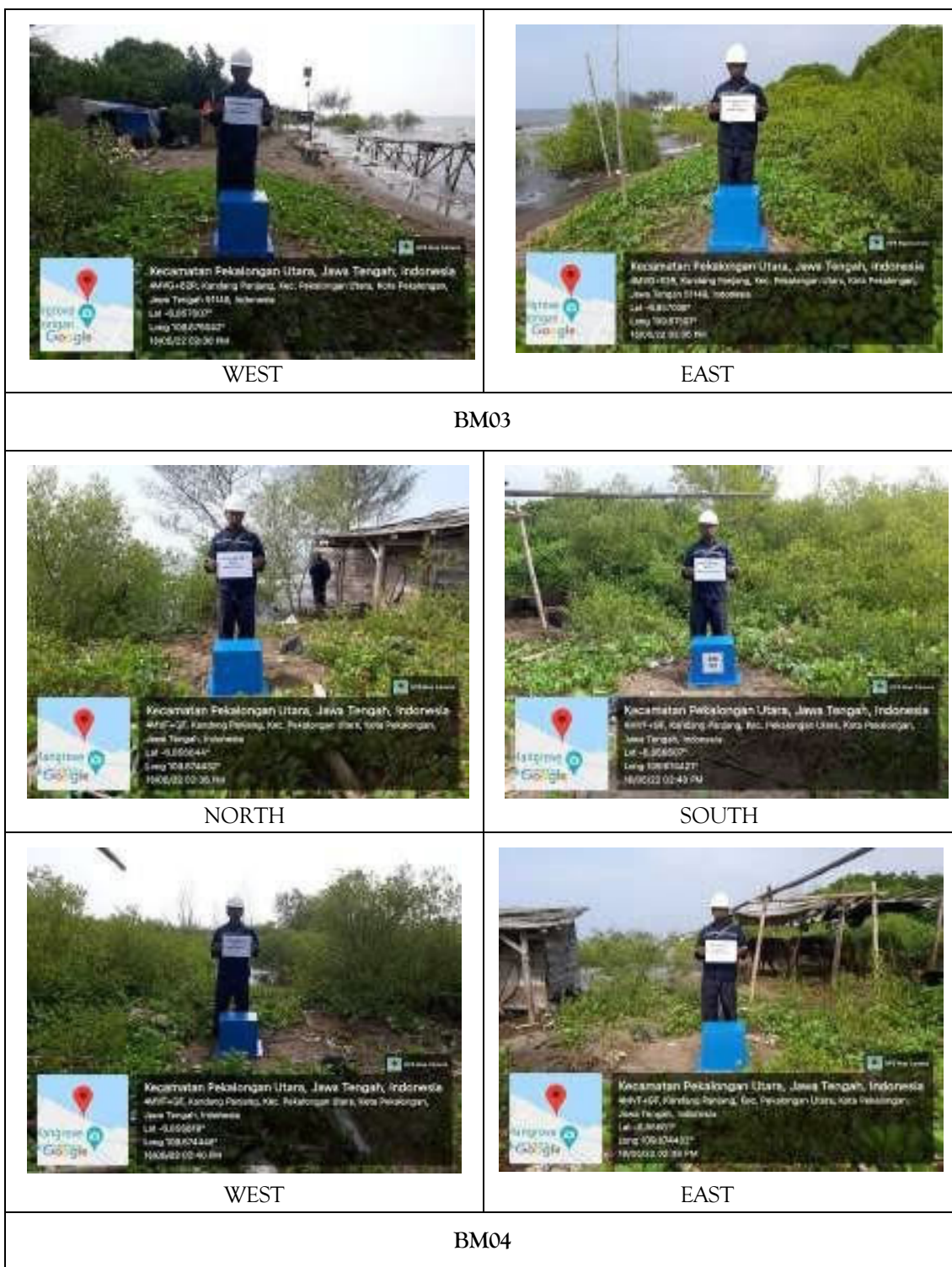
Figure 5.1 Results of making GPS01 and GPS02 Benchmarks in the Pekalongan Coastal Protection Study Area
