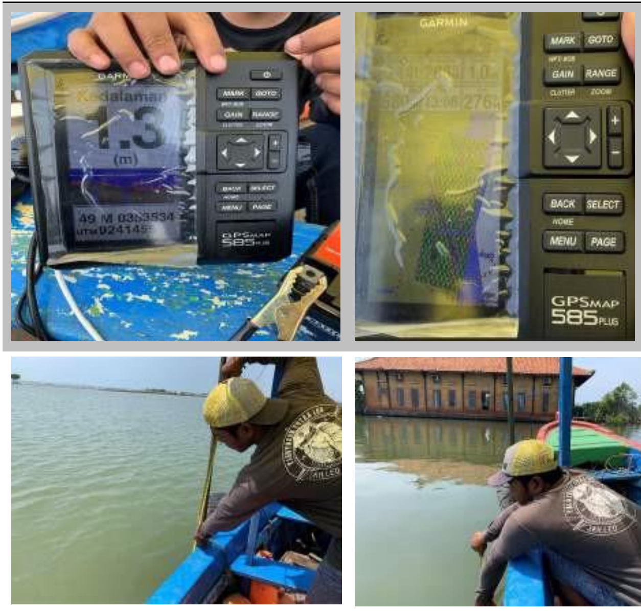
5.1.1.46 Figure 3.27 Documentation of bathymetric measurement and
