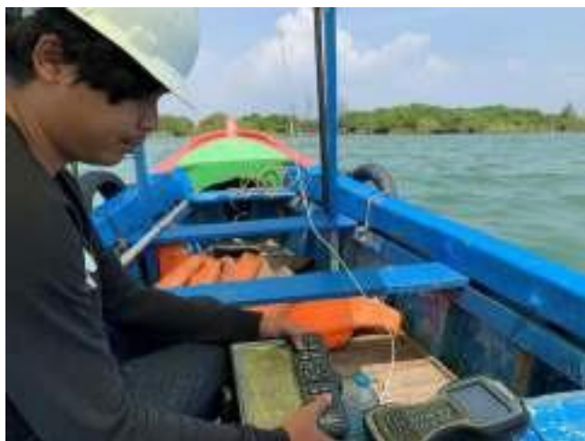
Figure 3.26 Snippet of the documentation of bathymetric measurement preparation with Echosounder 585
