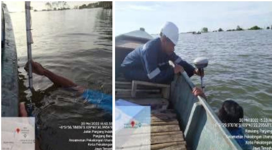
5.1.1.44 Figure 3.24 Snippet of the documentation of bathymetric measurement with the staff method
