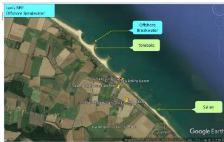
Figure 12 Example of separated offshore breakwater construction
