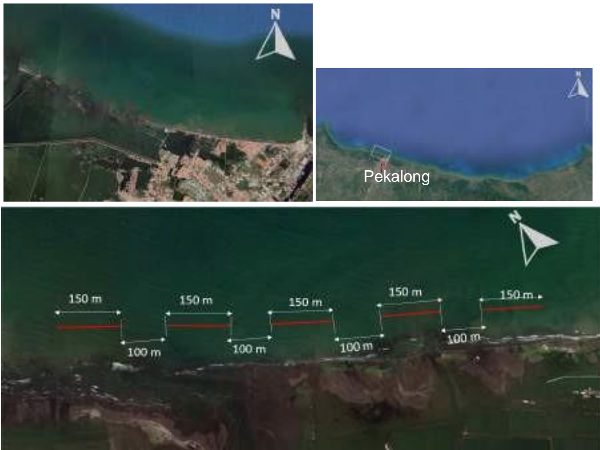
Figure 9.24 Details of the detached breakwater structure placement
