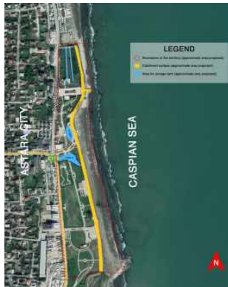
Figure 48: Caspian Sea Promenade, Astara City, Astara district, Azerbaijan: catchment surface and location for storage tanks (not to scale)
