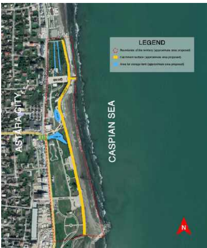
Figure 48: Caspian Sea Promenade, Astara City, Astara district, Azerbaijan: catchment surface and location for storage tanks (not to scale)
