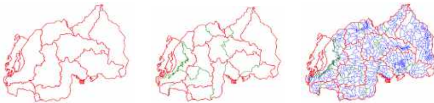
Figure 8: Levels of hydrologic analysis for Rwanda, with Level 1 on the left, Level 2 in the middle and Level 3 on the right. Source: VCRP Documents
