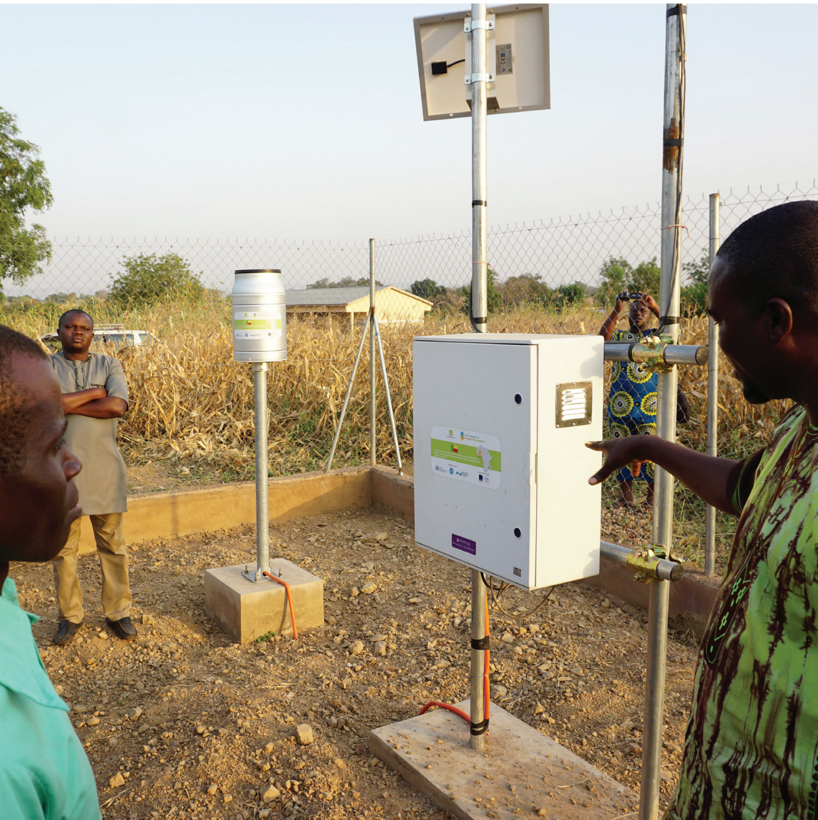
Meteorology and hydrology specialist explains how weather station gathers data, an AF-funded project to reduce disaster risks in Benin Photo by Adaptation Fund
