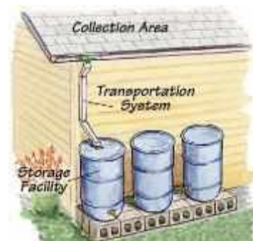
Figure 9 Conceptual diagram for rainwater harvesting system
