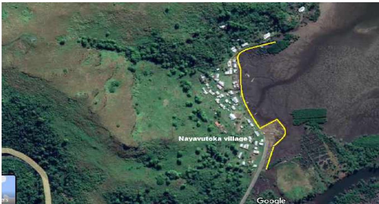
Figure 391: Proposed extent of Nayavutoka seawall.
