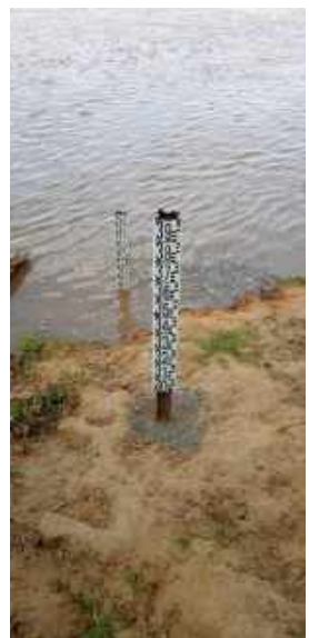
Water level gauge
