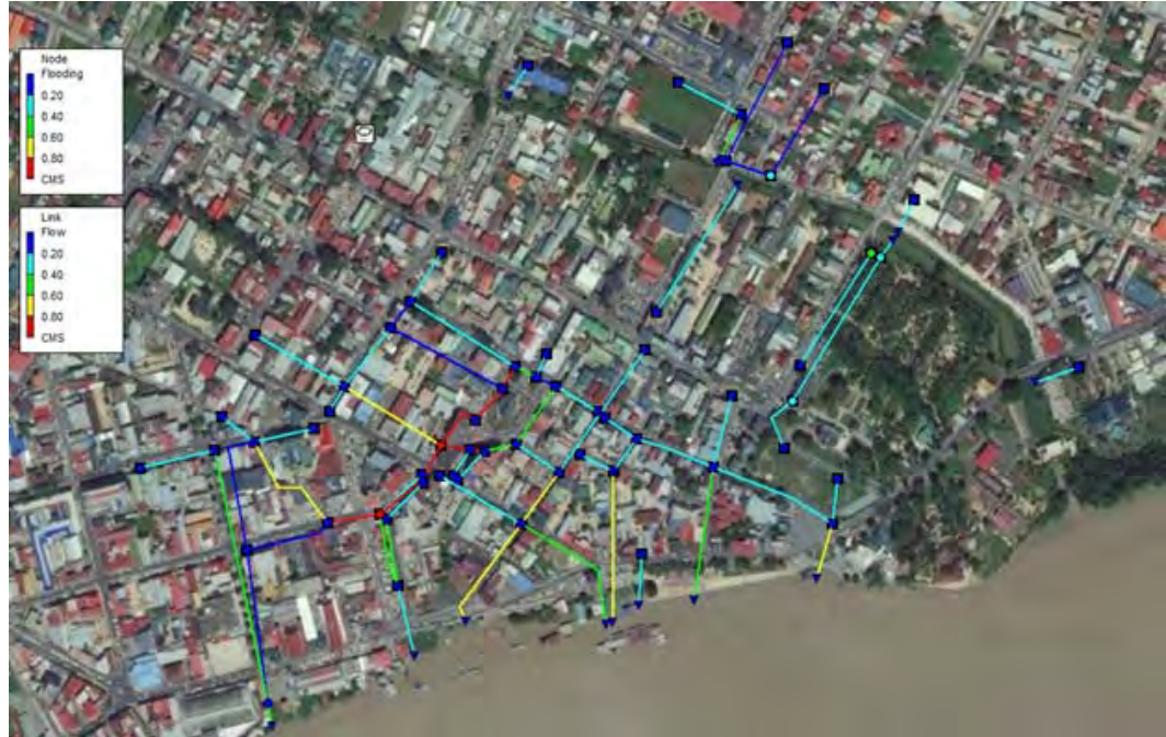
Figure 34: Pipe flow and inlet flooding for a baseline 100-year event. Flow rate in cubic meters per second (CMS)
