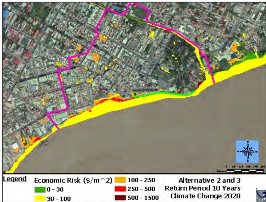
Figure 103: Economic-based risk map of the Study Area with the Alternative 2 and 3 conceptual designs for the climate change 2020 scenario at 10-year return period
