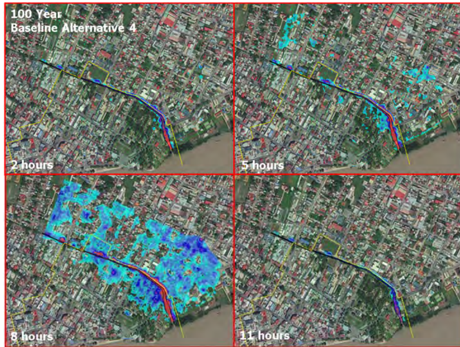
Figure C2- 11: Flooding inundation map of the Canal and its surroundings for Alternative 4 option and baseline scenario at 100-year return period
