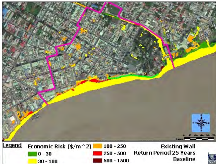
Figure 68: Economic-based risk map of the Study Area for the baseline scenario at 25-year return period
