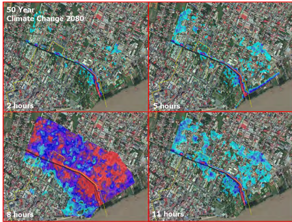
Figure C1- 32: Flooding inundation map of the Canal and its surroundings at discrete hours during the simulation of the climate change 2050 scenario at 50-year return period
