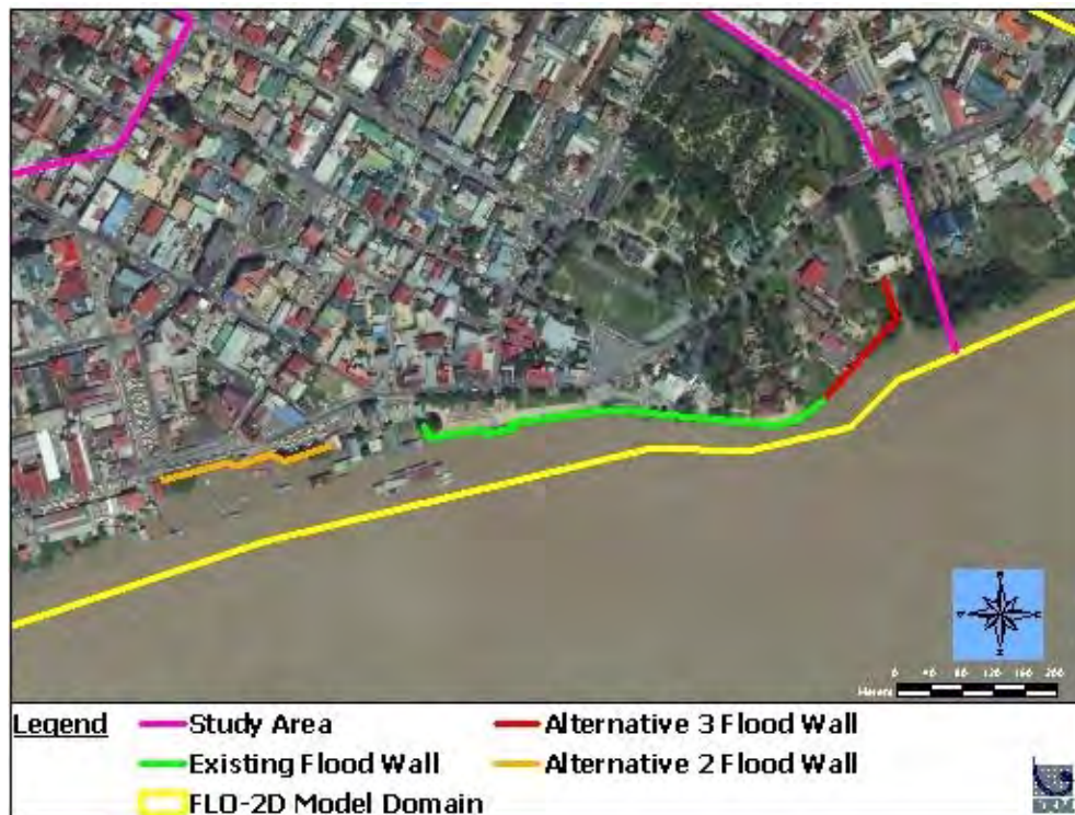
Figure B- 1: Alternative 2 and 3 conceptual design layouts on either side of the existing flood wall
