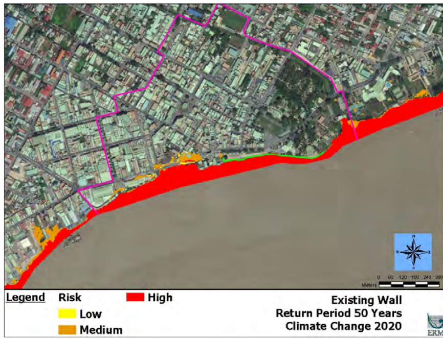
Figure A1- 18: Coastal flooding hazard map of the Study Area with the existing flood wall for the climate change 2020 scenario at 50-year return period
