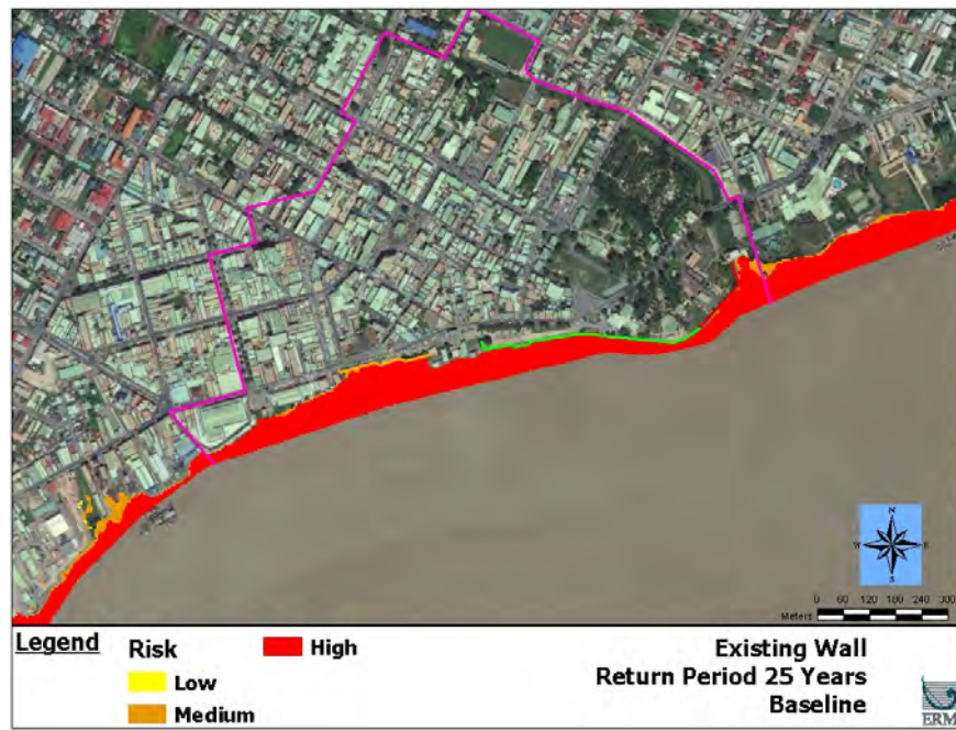
Figure B- 8: Coastal flooding hazard map of the Study Area with the Alternative 2 and 3 conceptual designs for the baseline scenario at 25-year return period
