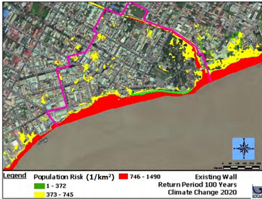
Figure 90: Population-based risk map of the Study Area for the climate change 2020 Scenario at 100-year return period
