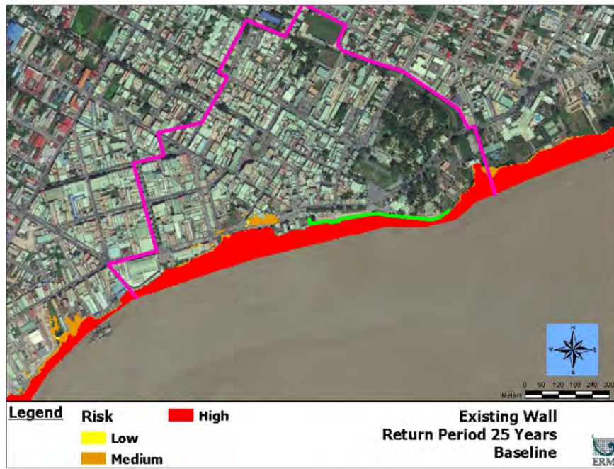
Figure A1- 7: Coastal flooding hazard map of the Study Area with the existing flood wall for the baseline scenario at 25-year return period
