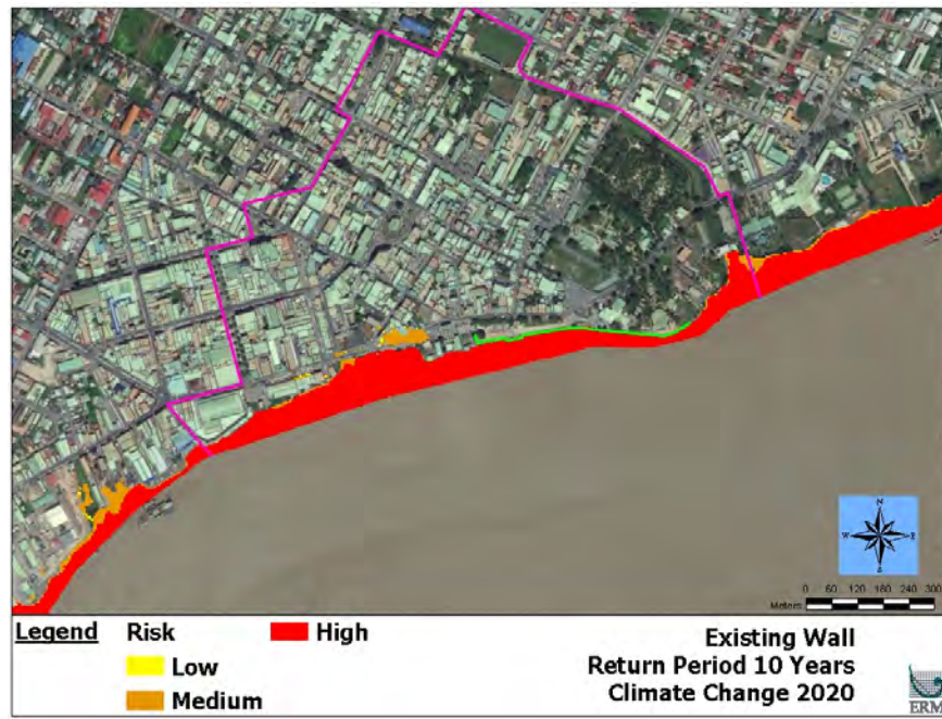
Figure A1- 16: Coastal flooding hazard map of the Study Area with the existing flood wall for the climate change 2020 scenario at 10-year return period
