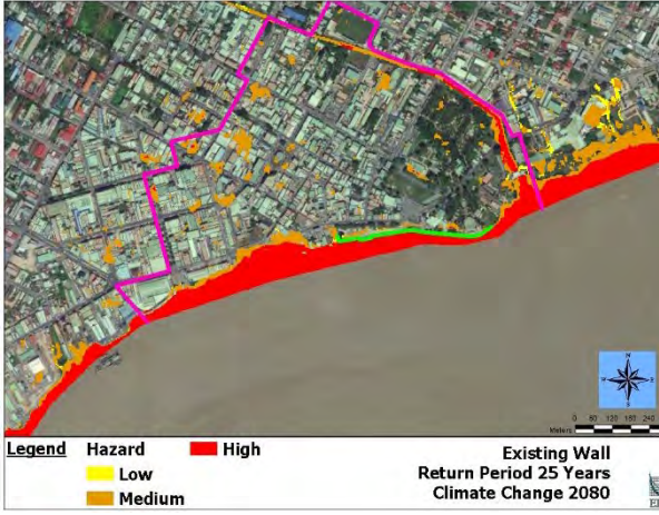
Figure 11: Coastal and inland flooding hazard map of the Study Area with the existing flood wall for the climate change 2080 scenario at 25-year return period
