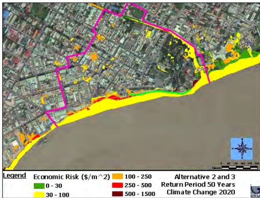
Figure 105: Economic-based risk map of the Study Area with the Alternative 2 and 3 conceptual designs for the climate change 2020 scenario at 50-year return period
