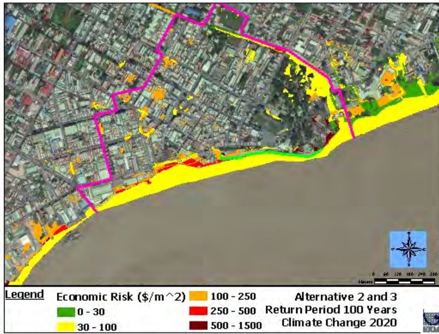
Figure 106: Economic-based risk map of the Study Area with the Alternative 2 and 3 conceptual designs for the climate change 2020 scenario at 100-year return period
