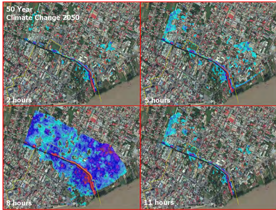
Figure C1- 21: Flooding inundation map of the Canal and its surroundings at discrete hours during the simulation of the climate change 2050 scenario at 50-year return period
