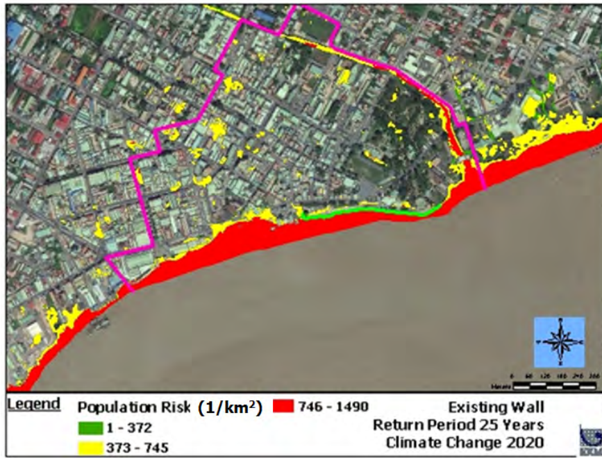
Figure 88: Population-based risk map of the Study Area for the climate change 2020 Scenario at 25-year return period
