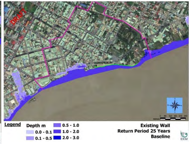
Figure 13: Coastal flooding inundation map of the Study Area with the existing flood wall for the baseline scenario at 25-year return period
