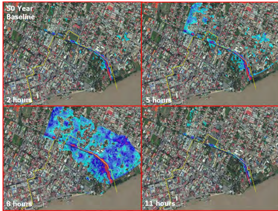
Figure C1- 10: Flooding inundation map of the Canal and its surroundings at discrete hours during the simulation of the baseline scenario at 50-year return period
