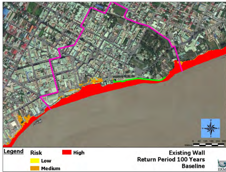
Figure A1- 9: Coastal flooding hazard map of the Study Area with the existing flood wall for the baseline scenario at 100 year return period
