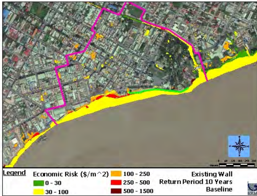
Figure 67: Economic-based risk map of the Study Area for the baseline scenario at 10-year return period
