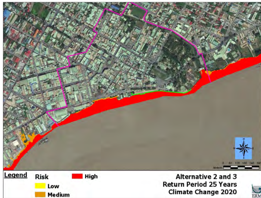
Figure B- 18: Coastal flooding hazard map of the Study Area with the Alternative 2 and 3 conceptual designs for the climate change 2020 scenario at 25-year return period
