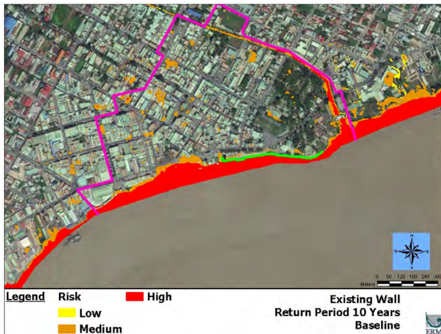
Figure A2- 6: Inland flooding hazard map of the Study Area with the existing flood wall for the baseline scenario at 10-year return period
