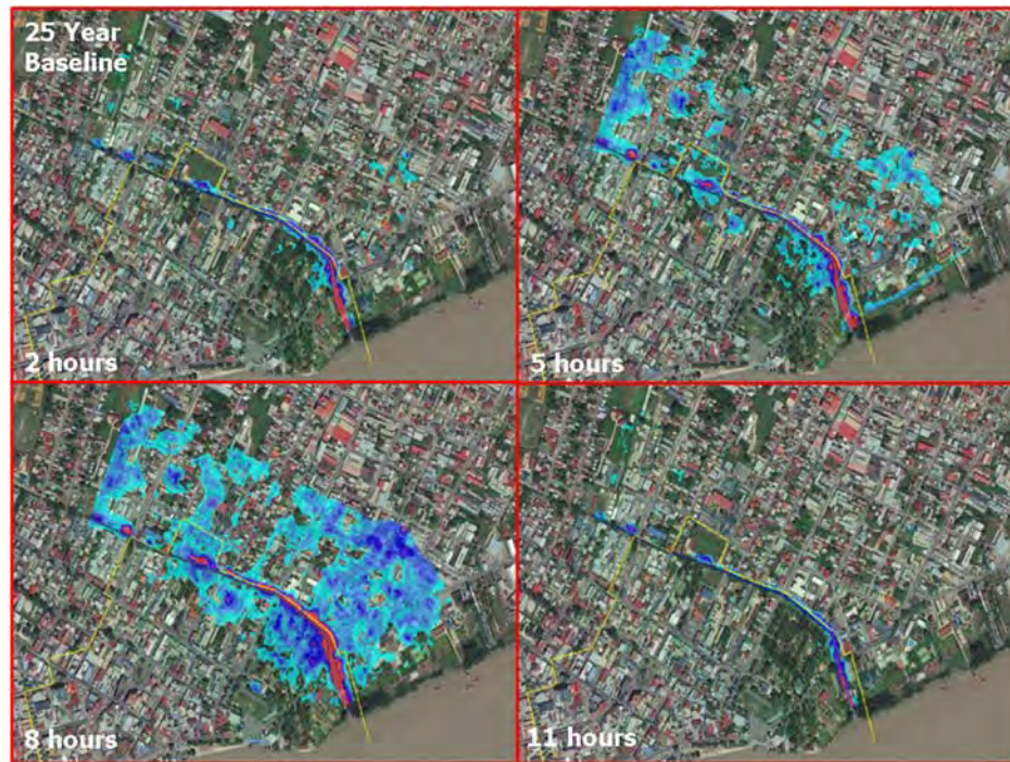
Figure C1- 9: Flooding inundation map of the Canal and its surroundings at discrete hours during the simulation of the baseline scenario at 25-year return period
