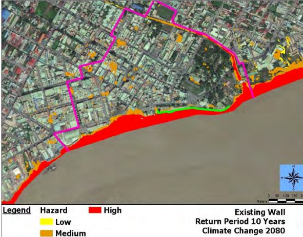
Figure 10: Coastal and inland flooding hazard map of the Study Area with the existing flood wall for the climate change 2080 scenario at 10-year return period
