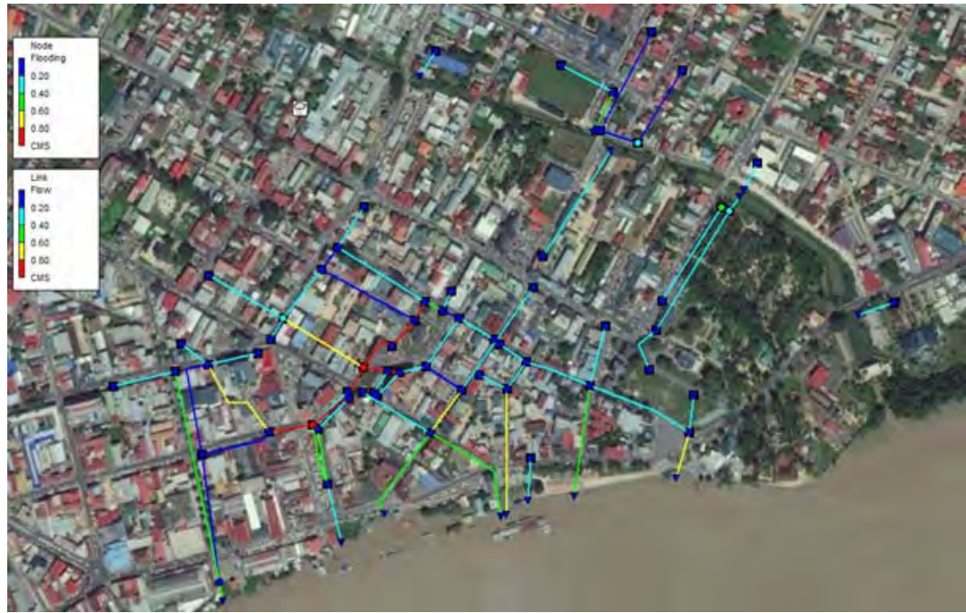
Figure 33: Pipe flow and inlet flooding for a baseline 50-year event. Flow rate in cubic meters per second (CMS)
