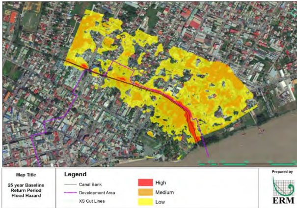
Figure 23: Flooding hazard map of the Canal and its surroundings for the climate change 2080 scenario at 25-year return period
