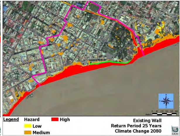
Figure 20: Coastal and inland flooding hazard map of the Study Area with the existing flood wall for the climate change 2080 scenario at 25-year return period
