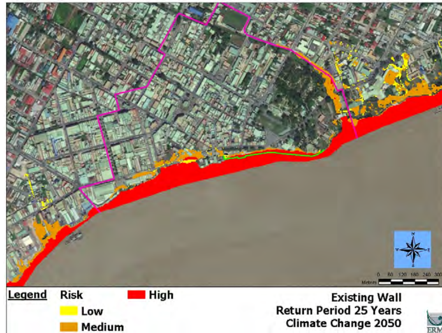
Figure A1- 27: Coastal flooding hazard map of the Study Area with the existing flood wall for the climate change 2050 scenario at 25-year return period
