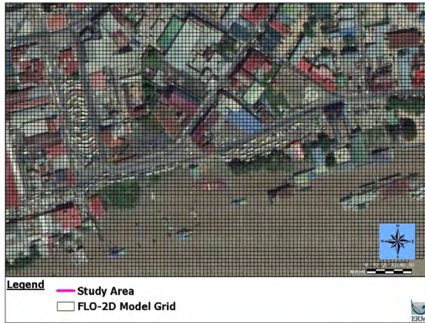
Figure 28: 4 m grid cell resolution at the waterfront capturing all details of the buildings in the Study Area
