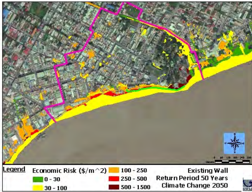
Figure 77: Economic-based risk map of the Study Area for the climate change 2050 scenario at 50-year return period
