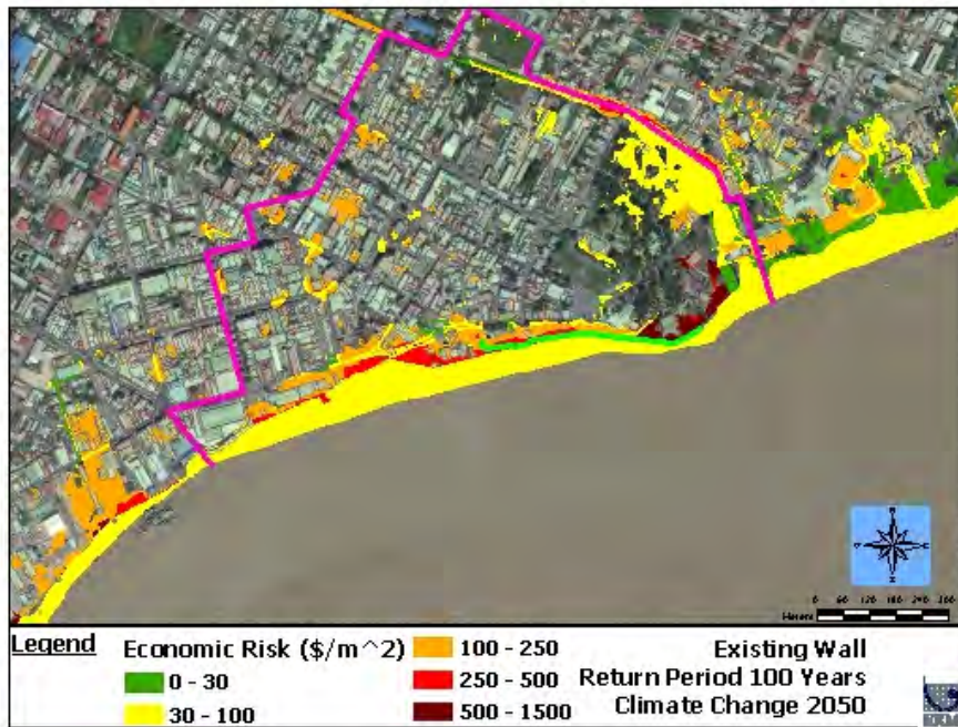
Figure 78: Economic-based risk map of the Study Area with the climate change 2050 scenario at 100-year return period
