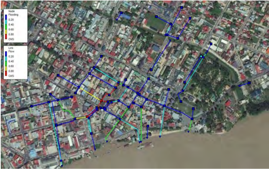
Figure 31: Pipe flow and inlet flooding for a baseline 10-year event. Flow rate in cubic meters per second (CMS)
