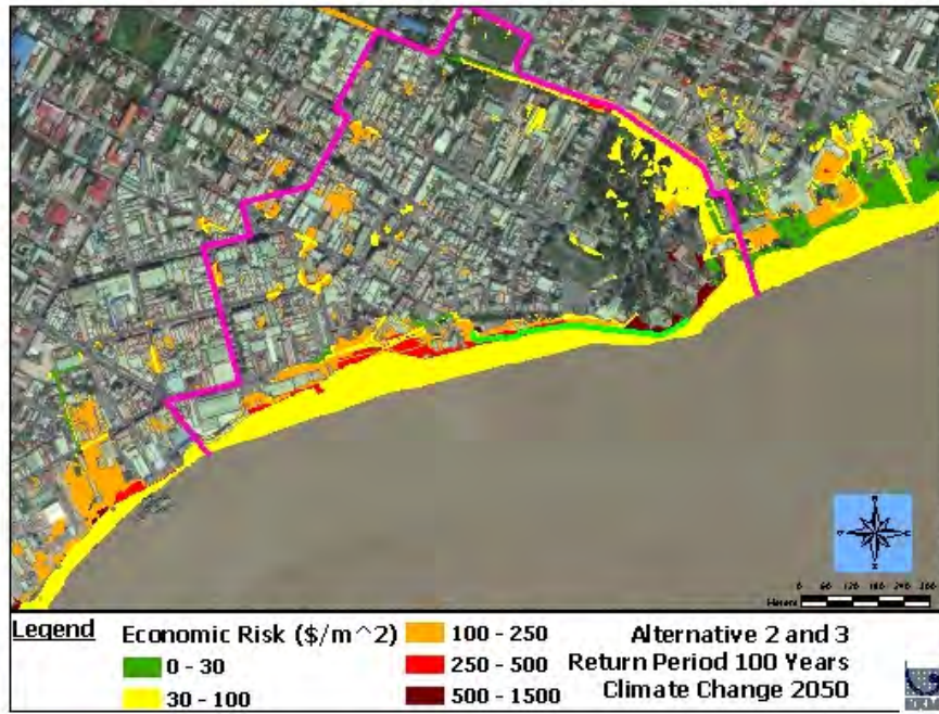
Figure 110: Economic-based risk map of the Study Area with the Alternative 2 and 3 conceptual designs for the climate change 2050 scenario at 100-year return period
