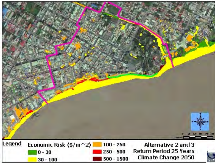
Figure 108: Economic-based risk map of the Study Area with the Alternative 2 and 3 conceptual designs for the climate change 2050 scenario at 25-year return period
