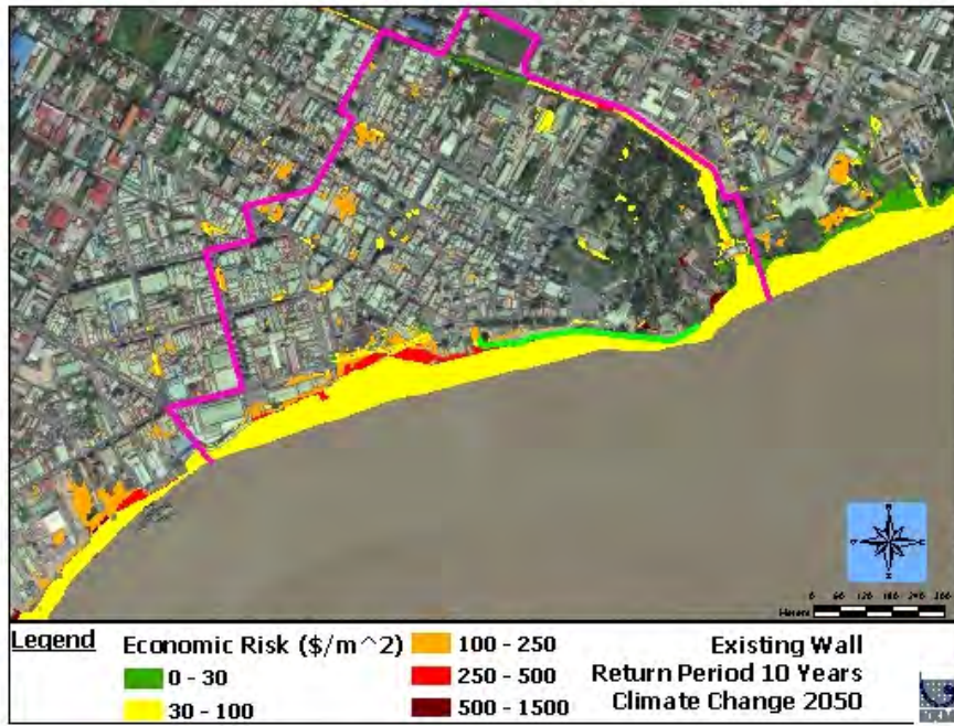
Figure 75: Economic-based risk map of the Study Area for the climate change 2050 scenario at 10-year return period
