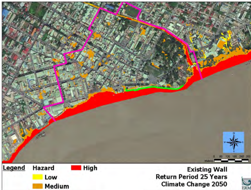
Figure A2- 17: Inland flooding hazard map of the Study Area with the existing flood wall for the climate change 2050 scenario at 25-year return period
