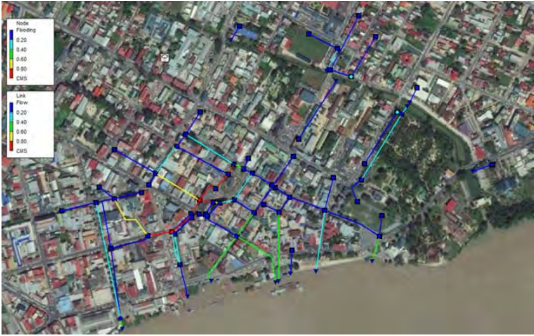
Figure 32: Pipe flow and inlet flooding for a baseline 25-year event. Flow rate in cubic meters per second (CMS)
