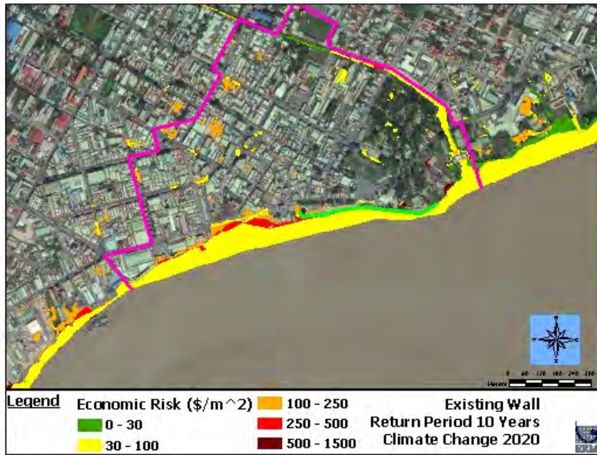
Figure 71: Economic-based risk map of the Study Area for the climate change 2020 scenario at 10-year return period
