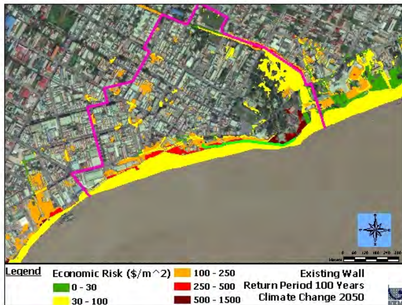
Figure 63: Economic-based risk map of the Study Area for the climate change 2050 scenario at 100-year return period
