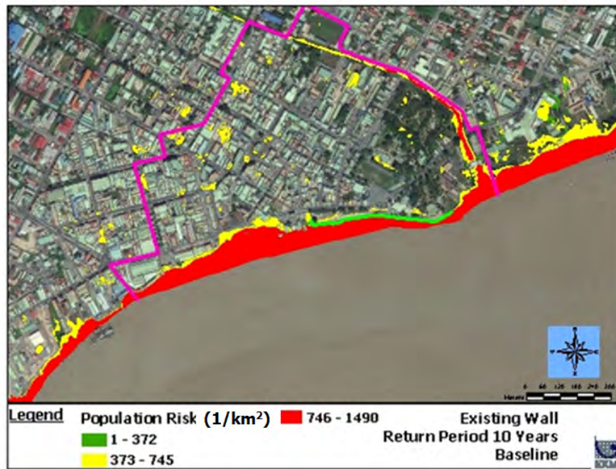
Figure 83: Population-based risk map of the Study Area for the baseline scenario at 10-year return period
