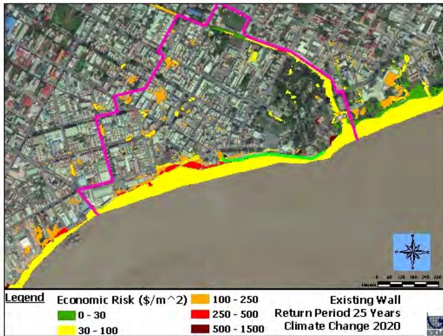
Figure 72: Economic-based risk map of the Study Area for the climate change 2020 scenario at 25-year return period
