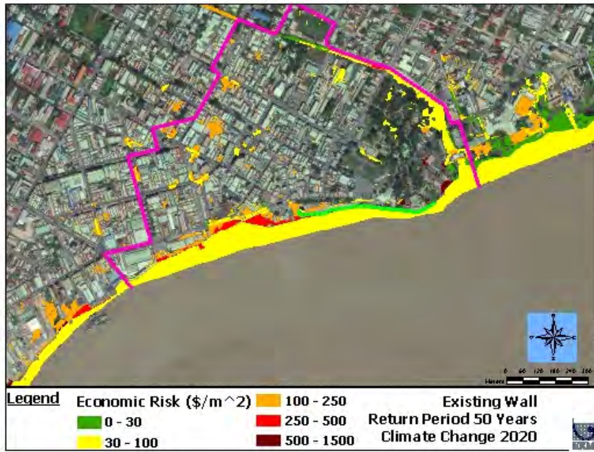
Figure 73: Economic-based risk map of the Study Area for the climate change 2020 scenario at 50-year return period
