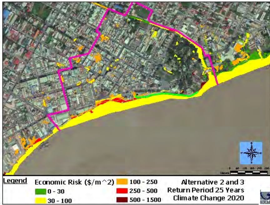
Figure 104: Economic-based risk map of the Study Area with the Alternative 2 and 3 conceptual designs for the climate change 2020 scenario at 25-year return period
