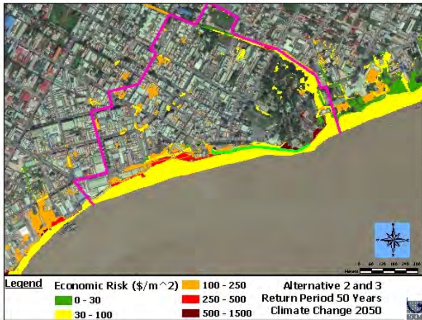
Figure 109: Economic-based risk map of the Study Area with the Alternative 2 and 3 conceptual designs for the climate change 2050 scenario at 50-year return period
