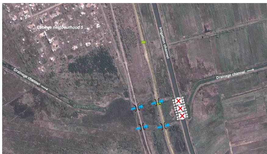
Figure 34: Detail of crossing "2" where the pipes going under the irrigation channel are collapsed
