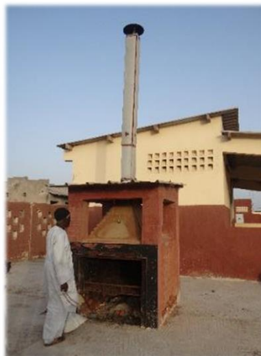
Photo 6. Prototype of a fish smoking kiln used for tests.
